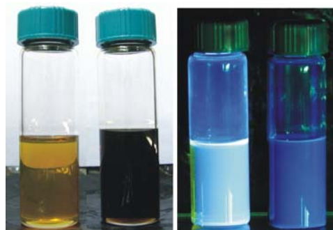
Fig. 1. Lubricating oil Titan Truck Plus 15W40 - fresh and used (593 h) - in visible light (left) and in ultraviolet (right)
