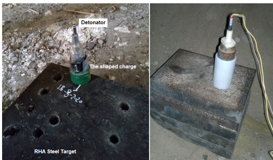
Figure 4. Ballistic test setup of the constructed shaped charges and the testing facility
