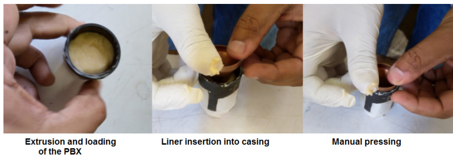
Figure 3. The explosive loading and the liner assembly (hydraulic pressing step not shown)
