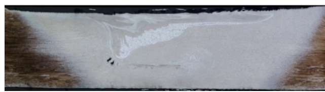
Fig. 8. Structure of FSW weld in the case of locating the rod of EN AC-43200 (A) on the advancing side. Welding parameters: \omega = 900 \text{ min}^{-1} , V = 224 \text{ mm/min} . Triflute pin. Etching: Keller
