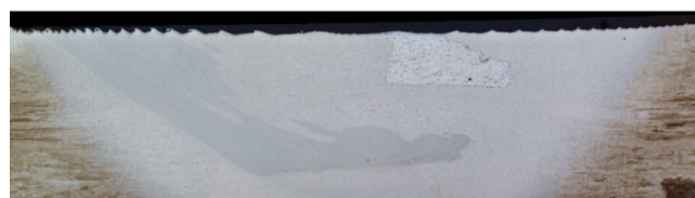
Fig. 7. Structure of FSW weld in the case of locating the rod of EN AC-43200 (A) on the retreating side. Welding parameters: \omega = 450 \text{ min}^{-1} , V = 224 \text{ mm/min} . Triflute pin. Etching: Keller
