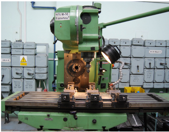
Fig. 2. Station for FSW welding process testing
