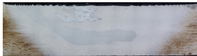
Fig. 6. Structure of FSW weld in the case of locating the rod of EN AC-43200 (A) on the advancing side. Welding parameters: \omega = 450 \text{ min}^{-1} , V = 224 \text{ mm/min} . Triflute pin. Etching: Keller
