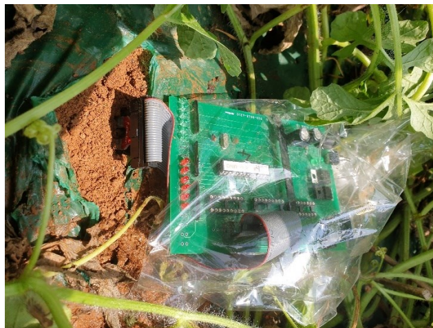
Figure 12. One of the tested moisture sensor modules inserted into the soil
