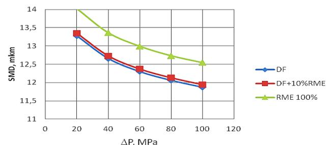
Fig. 2. Change of the average diameter of atomized fuel drop depending on the injected fuel pressure
