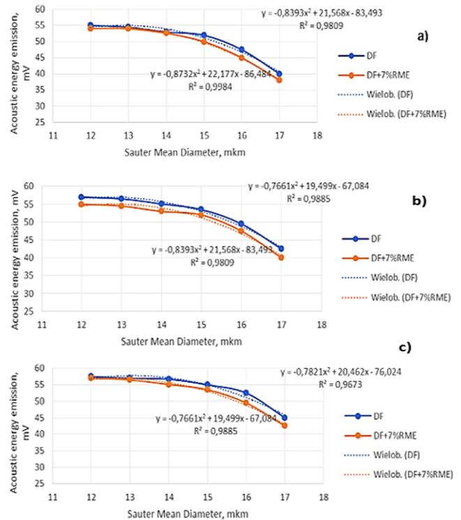
Fig. 10. Relationship between Sauter mean diameter of atomized fuel drop and level of the acoustic emission formed in the atomization process for the start fuel injection pressure: a – 22.0 MPa; b – 24.0 MPa; c – 26.0 MPa
