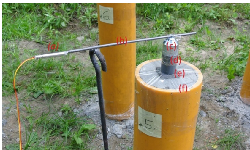
Figure 3. A view of a typical test arrangement, used for the steel-concrete target perforating ability test: electrical igniter (a), fragment of detonating cord (b), shaped charge (c), spacer (d), optional steel plate (e) and concrete core (f)
