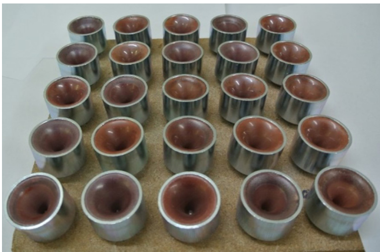
Figure 2. Experimental series of the tested elliptically shaped charges
