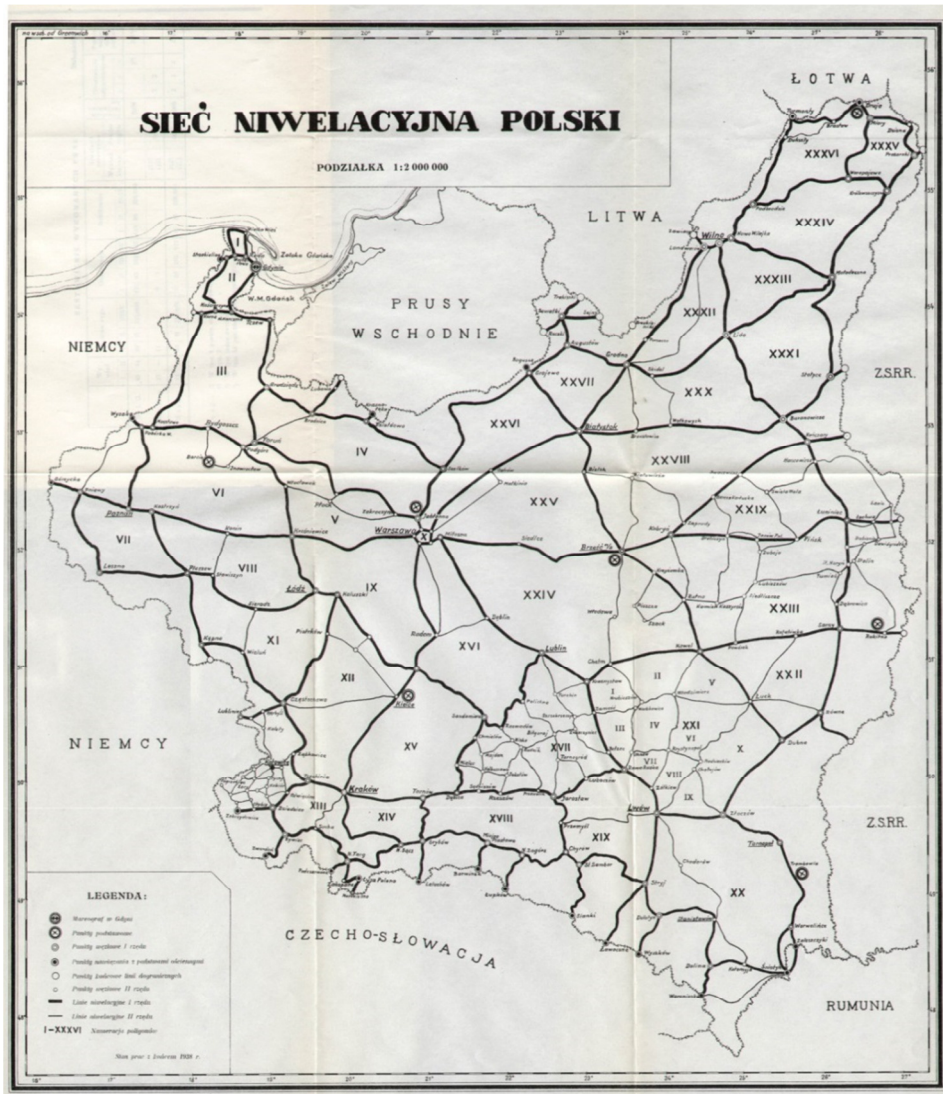
Fig. 1. Sketch of the basic height network during the times of the Second Polish Republic. According to the then naming, the network consisted of lines I and II order. Traverses closed numbered with Roman numerals. The age points (in the legend named as "basic") and a mareograph in Gdynia are marked by big circles. Source: Archive WIG [25]
