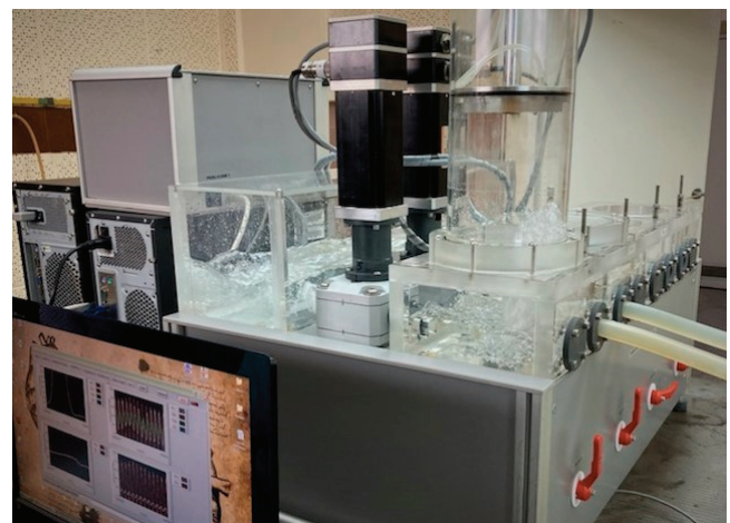
Fig. 1. The hybrid-digital model of the circulatory system
