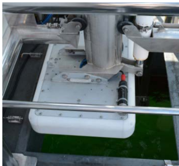
Figure 3. Hydrographic vessel and its multibeam transducer with a sound speed probe
