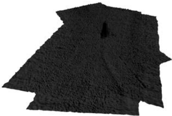
Figure 5. Visualization of the sea bottom obtained during hydrographic surveys using Coons surfaces
