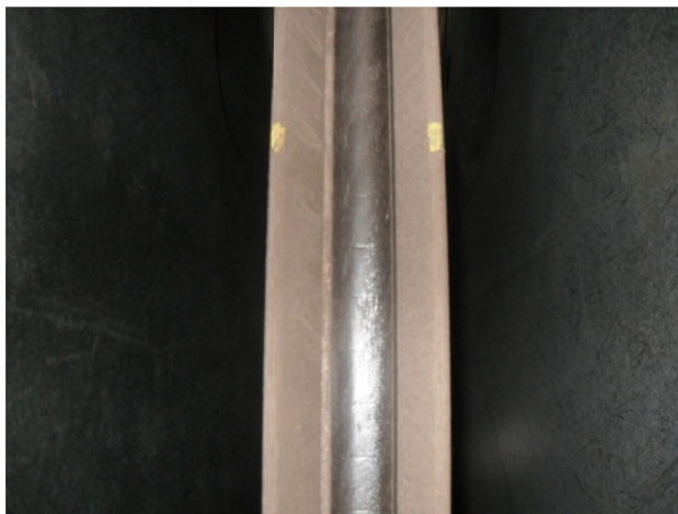
Fig. 3. Uneven wearing of the groove lining in a driving sheave (Nowacki & Tytko, 2011)
