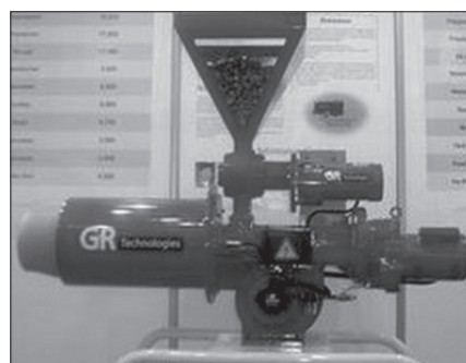
Fig. 2. Waste plastic burner: Combustion chamber: Burns PE or PP; PS & ABS require 50% barrel length increase. Rated capacity: 100,000 kcal/h on 9 kg/h with 11,500kcal/kg plastic fuel pellets. Plastic fuel feed rate range: 9÷15 kg/h. Current plastic fuel feed rate: 13 kg/h. Thermal efficiency: 75%; at 150°F water, thermal efficiency goes to 89%. Combustion chamber: 900÷1100°C. Boiler cut-in temperature: 60°C. Boiler cut-out temperature: 80°C. Boiler heating cycle: 5 h comprised of 2 h burning & 3 h circulating. Boiler heating rate: 1 ton water requires 45 minutes heating time (entire heating system will hold 3 tons water with 2 hours heating time). Power needs: 4 kW 110 vac with 208 vac for vacuum fuel supply. Future boiler: 2,000,000 kcal/h. [Manufacturer: GR Technologies Company, Ltd., Seoul, Korea. Specifications for the PENN STATE Agricultural Program, 2009]
