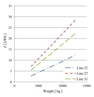
Fig. 11. Course of the energy required to pass the cycle E-50% occupation
