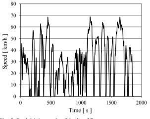
Fig. 5. Real driving cycle of the line 27
