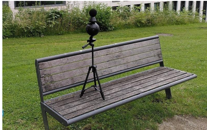
Figure 2. Recording Setting in the park, with an Insta360 Pro 2 and a Zoom H3-VR 1st order Ambisonics microphone.
