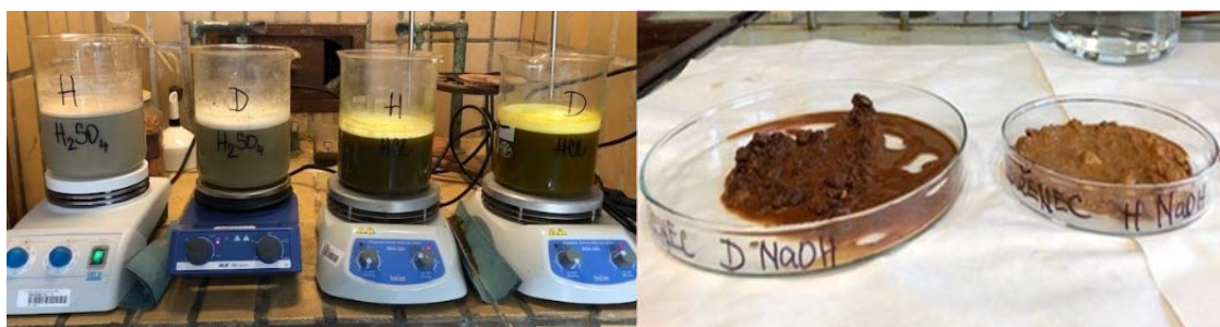
Fig. 1. Preparation of samples for leaching and the leaching process
