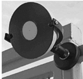
Fig. 5. Circular flat target combined with hemispherical shape by Leica [8].
