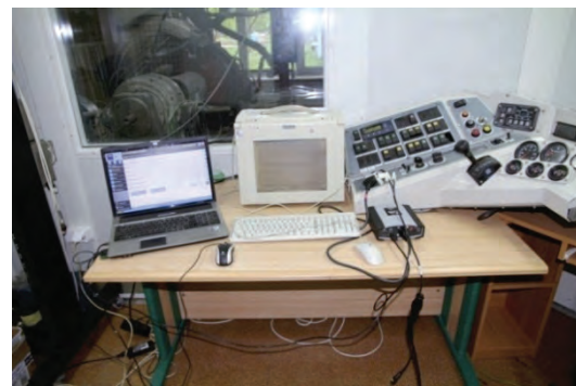
Fig. 2. Test stand for test drive units AMV Rosomak: a) the engine with the gearbox, in the back can see the control cabin, b) diagnostics device TEXA with computer and driver's console (Source: by authors)
