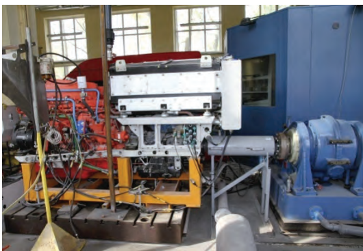
Fig. 2. Test stand for test drive units AMV Rosomak: a) the engine with the gearbox, in the back can see the control cabin, b) diagnostics device TEXA with computer and driver's console (Source: by authors)
