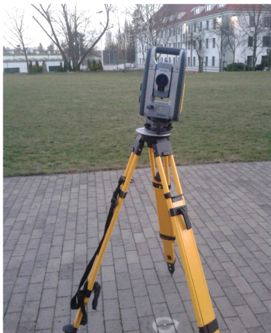
Fig. 3. Oblique tachymeter during surveying
