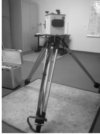
Figure 1. Vertical gravity gradient measurement on two levels
