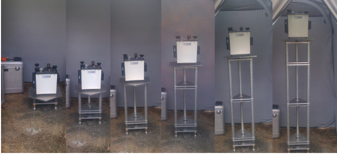
Figure 4. Vertical gradient measurement at 156 field station
