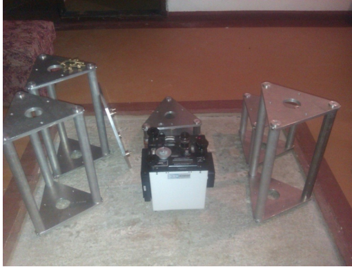
Figure 2. LaCoste&Romberg G-1012 with all segments of the stand
