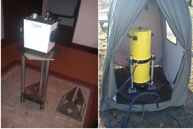
Figure 3. LCR G-1012 on the constructed stand (left) at A-BG station, A10 measurement at 156 field station (right)
