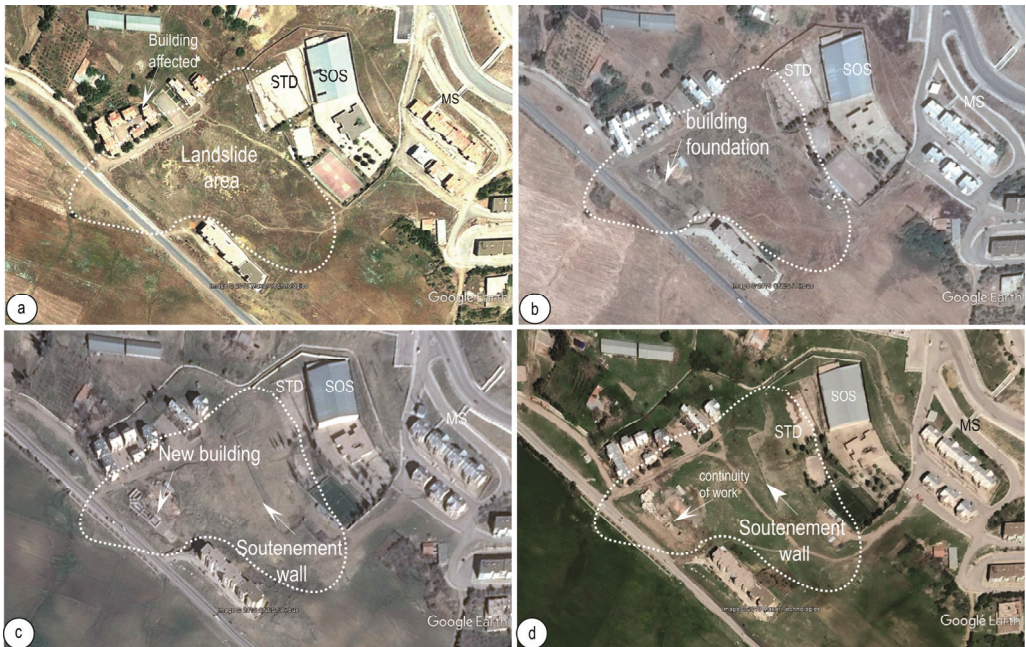
Fig. 5. Google earth quick looks showing the landslide area and also the anarchic work that lead to the installation of a multi-storey apartment building: a)–d) are different satellites images dating of 08/06/2010, 09/12/2012, 29/07/2013 and 20/02/2018, respectively.
