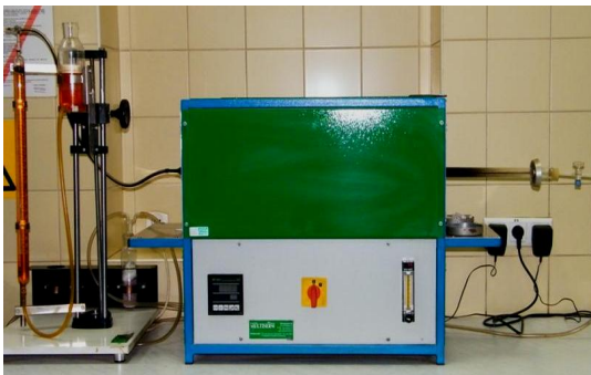
Fig. 1. Laboratory station for analysis of moulding mass gas generation properties
