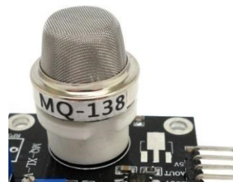
Fig. 5. MQ138 sensor Used to detect Nitrogen Dioxide
