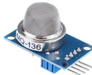
Fig. 4. MQ136 sensor Used to detect Sulfur Dioxide
