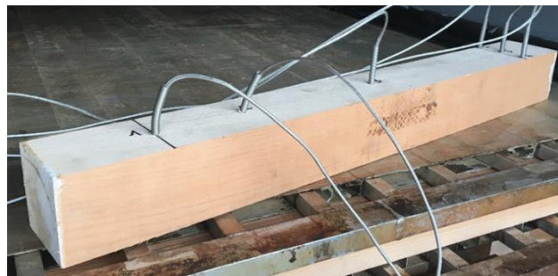
Figure 2. Beech frieze with sensors for temperature measurement
