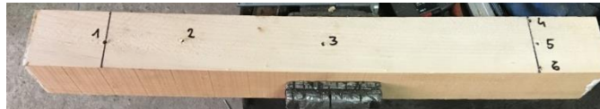
Figure 1. An element in the form of a beech frieze with designated places for measuring the temperature of the wood during the drying process
