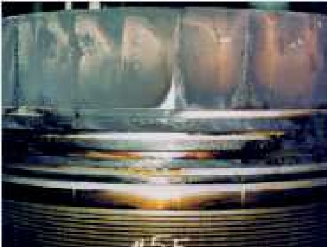
Fig. 2. View of damaged side surface of a piston due to its seizure in cylinder liner and breaking of sealing rings. [8, 23, 25]
