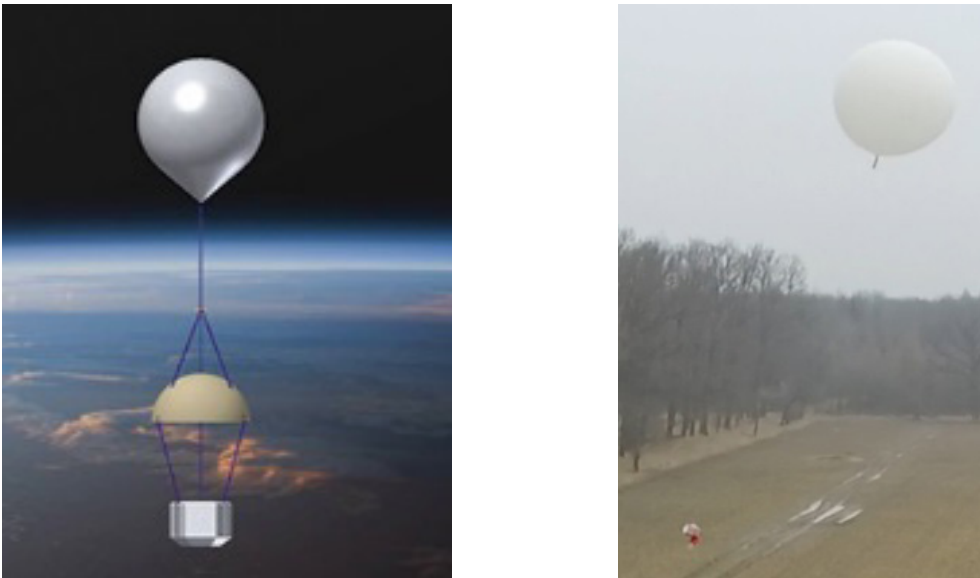
Fig. 2. a) The concept of connecting a gondola, parachute and balloon, which allows for the automatic activation of the parachute after cutting off the balloon [12], and b) the concept actually used in the mission - the balloon, regardless of the parachute, is permanently attached to the gondola.
