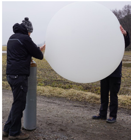
Fig. 4. Filling the balloon using helium cylinder at the HESOFF research area - Piaski Forest District.
