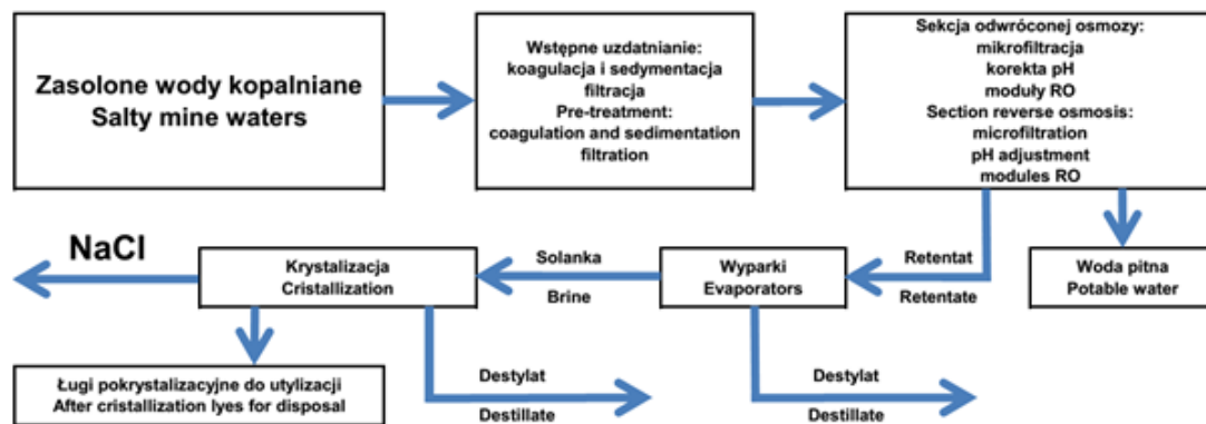
Fig. 4. Installation diagram for desalination of mine waters
