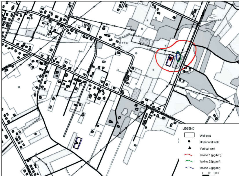
Fig. 5. Spatial distribution of NO 2 – maximum yearly NO x concentration during hydraulic fracturing
