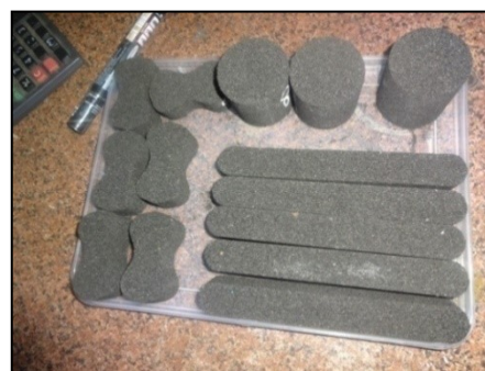
Fig. 3. Compressive, tensile and transverse test specimens
