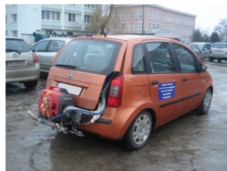
Fig. 1. Fiat Idea with mounted exhaust measuring apparatus [1]
