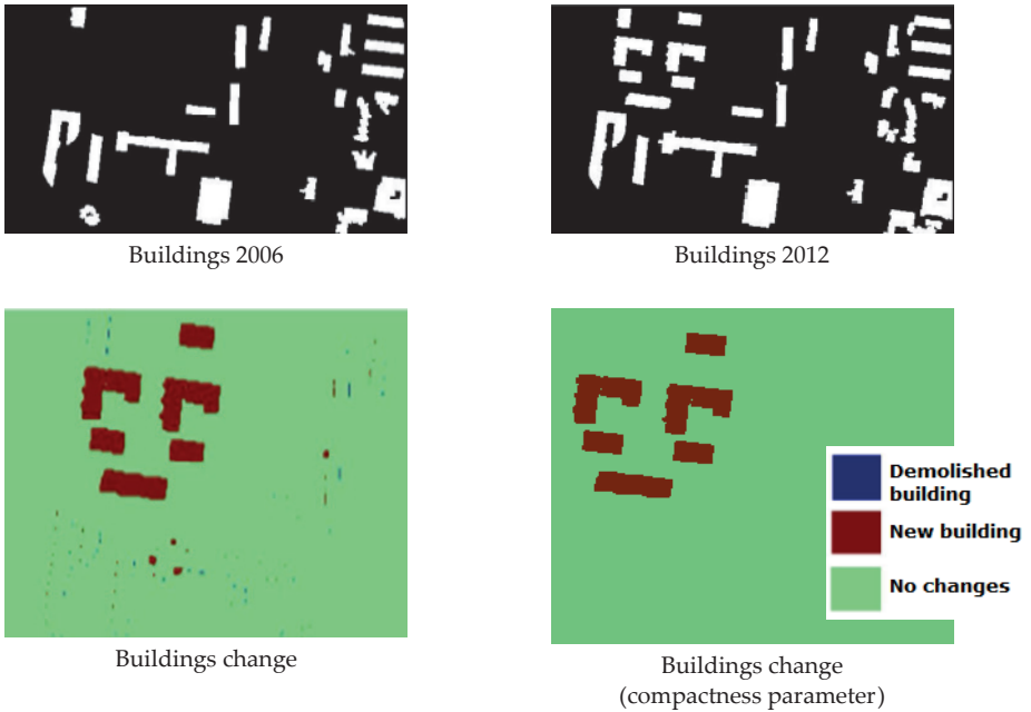
Fig. 4. The elimination of artifacts based on the compactness parameter
