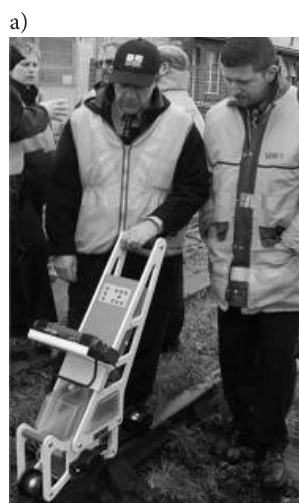
Fig. 3. Ultrasonic defectoscopy technique [11]
