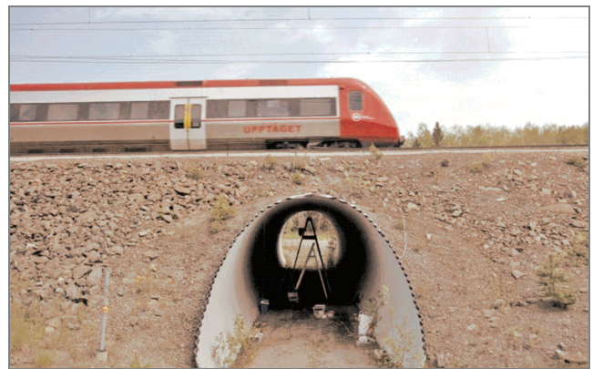
Fig. 1. The passage of a train along a soil-steel structure in a dynamic test [4]
