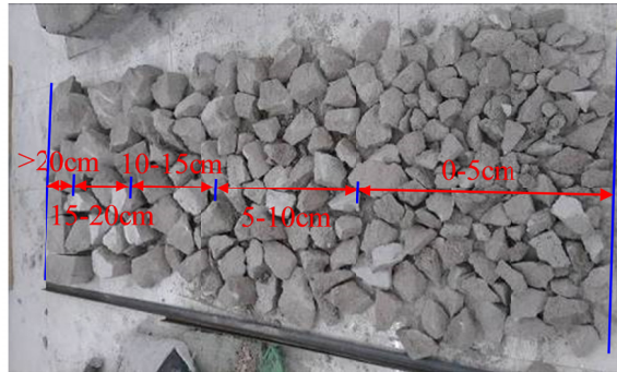
Fig. 4. Lumpiness of rock and coal fragments made from similar materials
