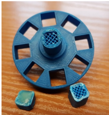
Fig. 15 Damaged rotor shaft of the single-row cylindrical clutch Source: [6].
