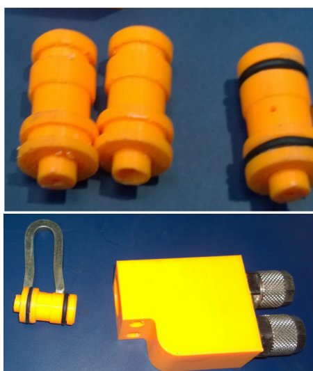
Fig. 8 Plug-in nozzle - 3 variants + complete feeding body
