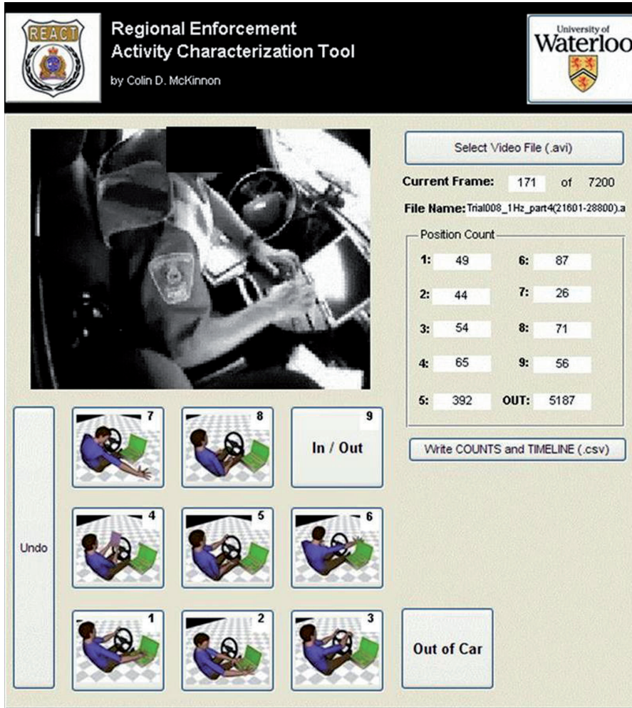
Figure 2. Regional Enforcement Activity Characterization Tool (REACT) graphical user interface for officer activity selection. Officer activity postures consider the entire body matched to one of the 10 postures shown for each frame of digital video.
