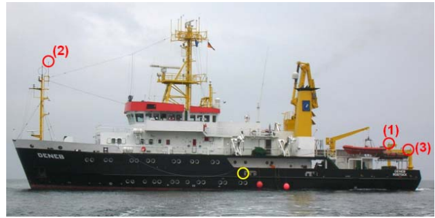
Figure 5. Vessel DENEK with sensor locations
