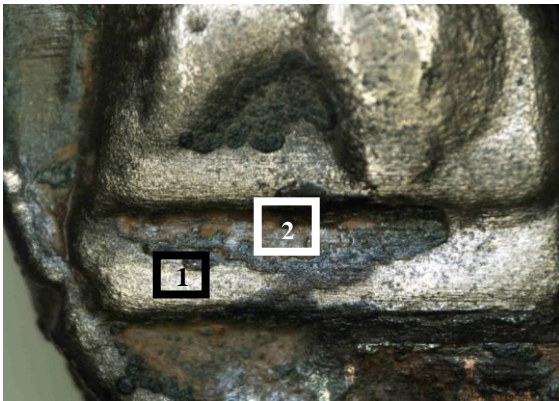
Picture. 8. Macroscopic picture, a visible area of missing cladding, during the conservation process.
