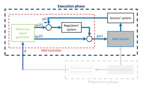
Fig. 2. Method of controlling an autonomous vehicle [4]
