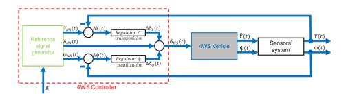
Fig. 15. Full structure of mechatronic control system [4]
