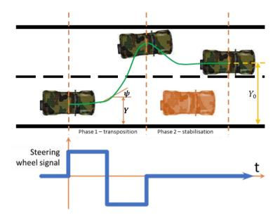
Fig. 12. Lane change process including control signal
