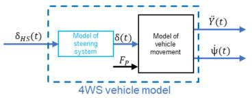
Fig. 13. Virtual 4WS vehicle [4]
