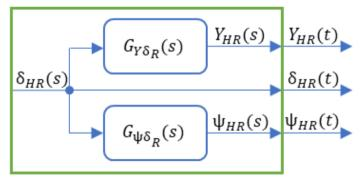
Fig. 11. Reference signal generator [4]
