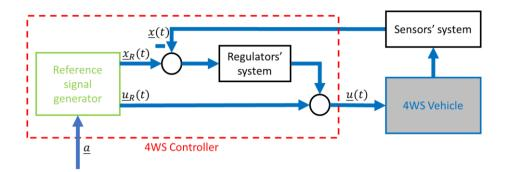
Fig. 4. Mechatronic control concept analysed
