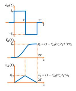
Fig. 10. Reference signals in the control system [4]
