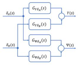
Fig. 6. Model in transfer function version [3]
