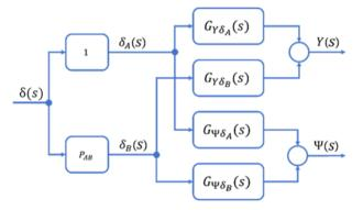
Fig. 8. Model including rear wheel ratio [3]
