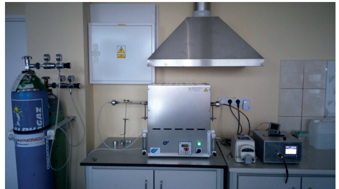
Fig. 1. Research stand for measuring the gas evolution rate of materials (acc. to Method 1), Laboratory of Environmental Protection
