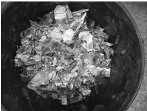
Fig. 3. Metallic contaminations separated from spent burned out sand
