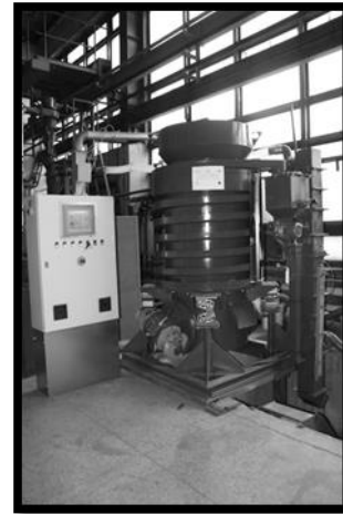
Fig. 4. View of the experimental reclaimer, at the background of the reclaim feeding system into the pneumatic classifier
