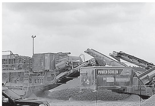
Figure 2. Limestone processing combine unit: crusher and vibrating sieve.
