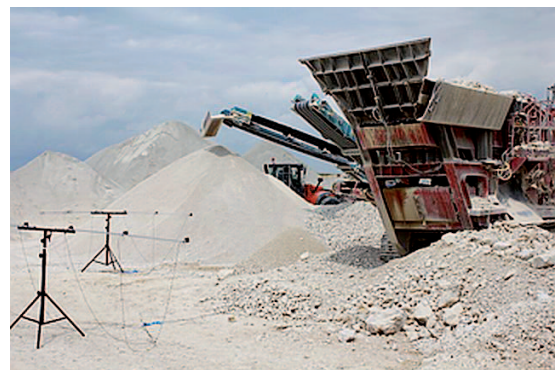
Figure 4. Arrangement of measuring microphones around the crusher.
