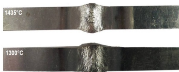
Fig. 14. Photos of samples compressed at temperatures of 1,300^{\circ}\text{C} and 1,435^{\circ}\text{C}
