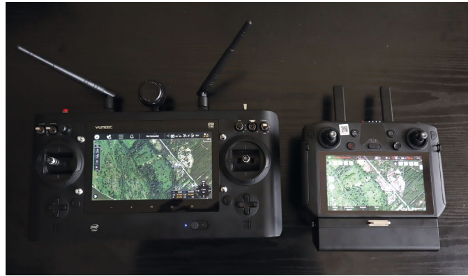
Figure 3. Comparison of the brightness of the screens of Yuneec Typhoon H520 ground stations (on the left, brightness approx. 400 cd/m 2 ) and DJI Matrice 300 (on the right, brightness up to 1000 cd/m 2 )
