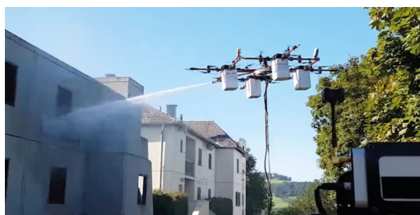
Figure 4. Examples of UAVs designed to extinguish fires: SKU: FFU-012, manufacturer UAVForDrone (on the left), firefighting drone, manufacturer AERONES (on the right)
