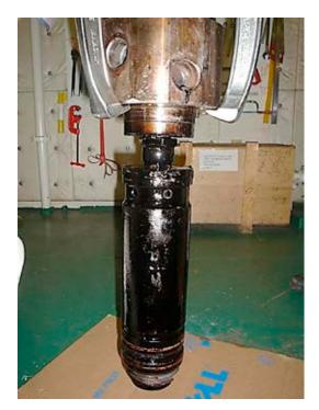
Figure 2. Dismantled barrel of fuel pump, unit No. 1 after failure
