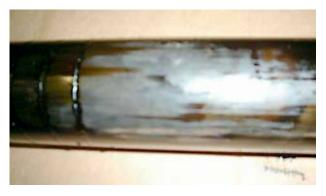
Figure 3. Traces of seizure on the fuel pump plunger, No. 1 unit after failure
