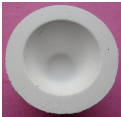
Figure 7. The new booster pellet (a). Figure 8. A cylindrical booster pellet.
