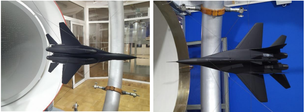
Photo 2. MiG-29 aircraft model during tests in the wind tunnel, with and without a rocket placed on the back
