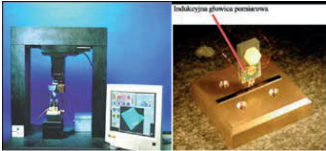
Rys. 22. Stanowisko BEMI – Barkhausen Eddy Current Microscope izfp
