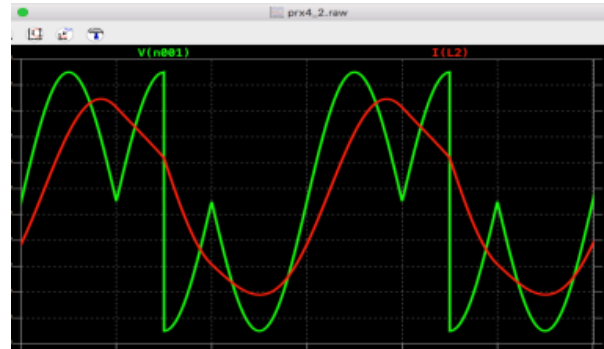
Fig. 10 Voltage and current waveforms of auxiliary phase with LC filter at 33.33 Hz
