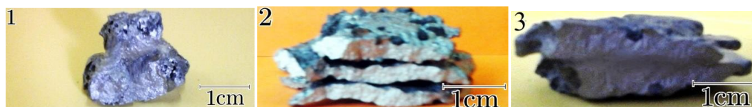
Fig. 7. Photographs of the obtained ferroalloys (fragments). 1 - 40% of C, 17% of St (41.3% of Si); 2 - 40% of C, 35% of St (27.4% of Si); 3 - 30% of C, 40% of St (19.6% of Si)
