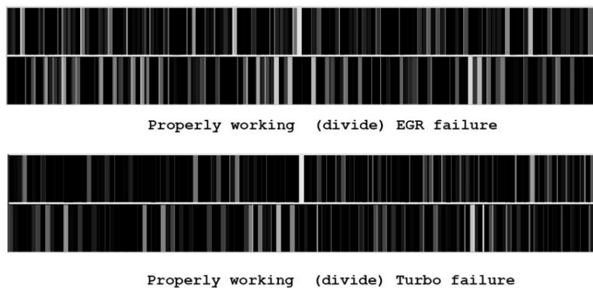
Fig. 7. The result of the application of the graphical divide function between the layers, being the results of the wavelet analysis; black indicates the places that differ
