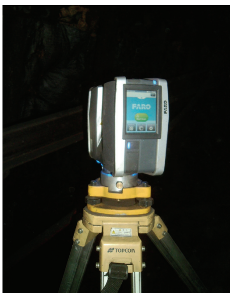
Fig. 3. The FARO Focus 3D scanner during operation
